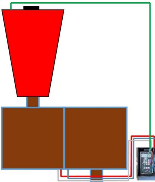
Figure 14: Recording of the differential pressures with simulation of the wind pressure through the fan
