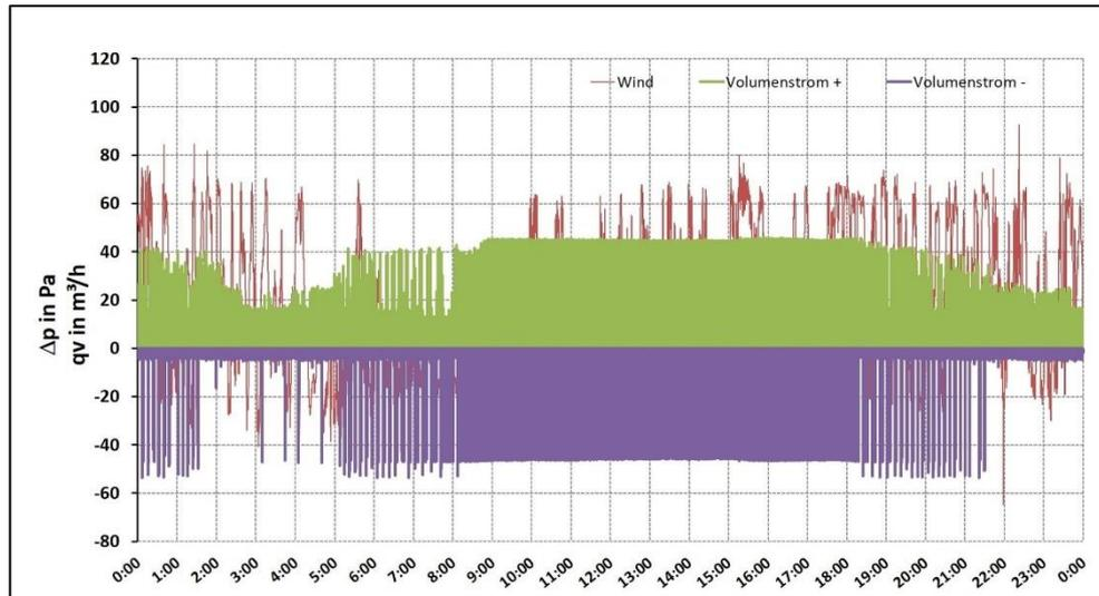
Figure 6: Effective wind pressure (red), volume flow measured via the orifice in delivery direction 1 (green) and delivery direction 2 (violet) at operating level 4: 21/3/18
