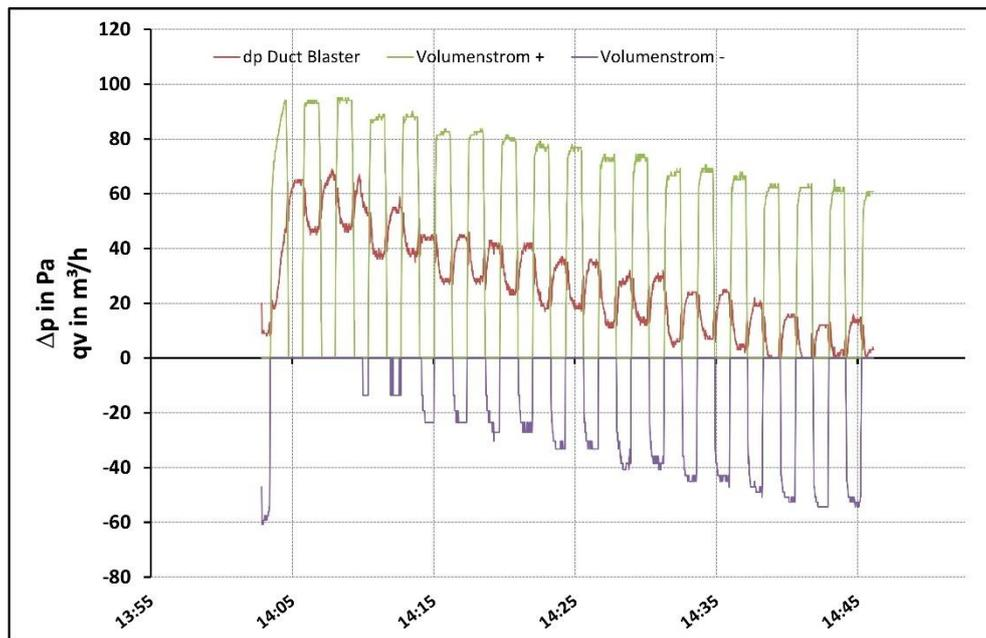
Figure 15: Volume flow under simulated wind pressure: Level 4,  $q_{v,target} = 58 \text{ m}^3/\text{h}$
