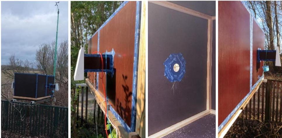
Figure 3: Measurement setup of the ventilation units operating in pairs
