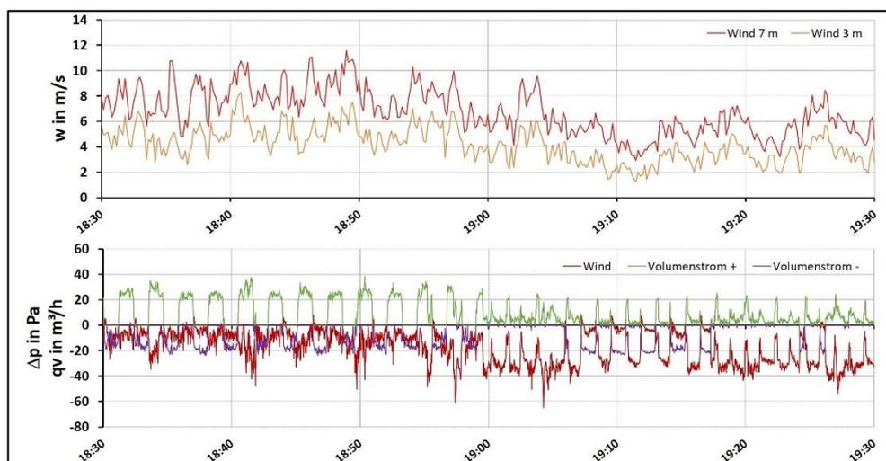
Figure 10: Wind speed at a height of 7 m (light red) and 3 m (dark red), effective wind pressure (red), volume flow measured via the orifice in delivery direction 1 (green) and delivery direction 2 (violet) at operating level 3 from 21/4/5, 6.30 to 7.30 p.m.
