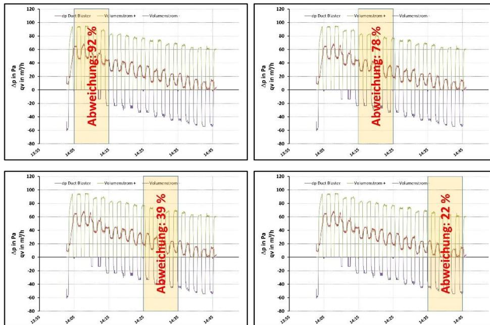
Figure 19: Percentage deviation of the supply air volume flow (green) from the extract air volume flow (violet) summarised in pressure bands at different simulated wind pressures (red) at operating level 4
