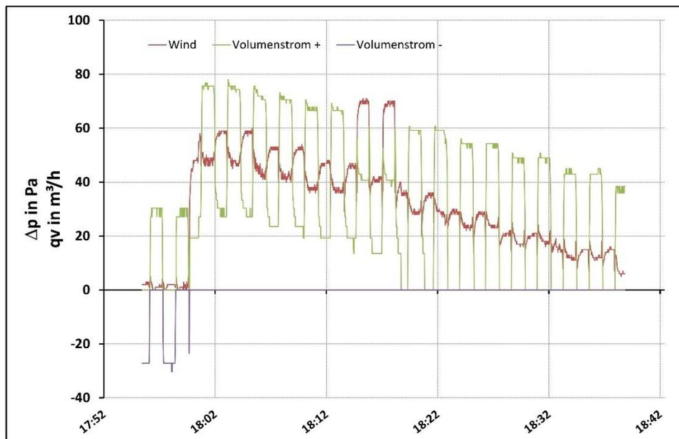
Figure 16: Volume flow under simulated wind pressure: Level 3,  $q_{v,target} = 42 \text{ m}^3/\text{h}$
