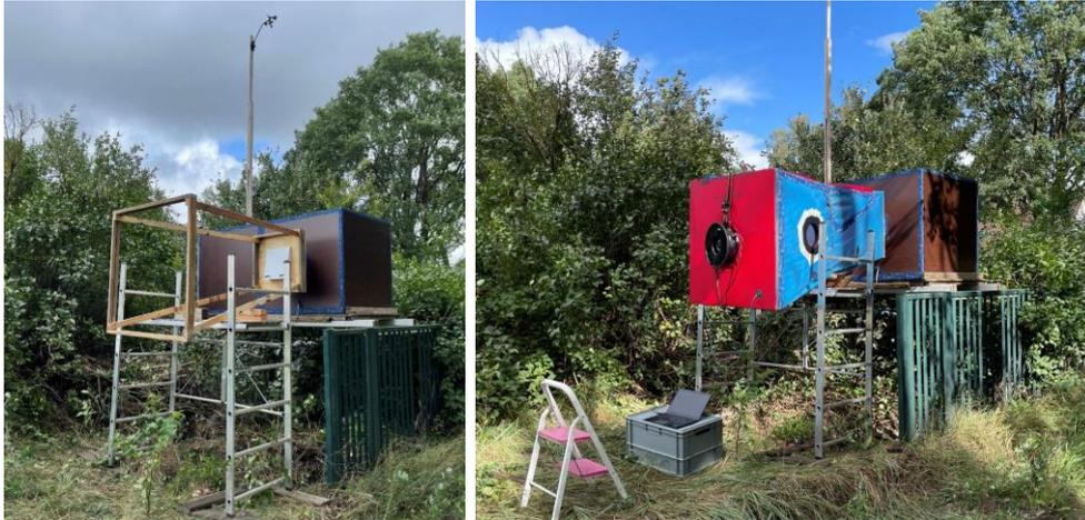
Figure 13: Measurement setup with fan to simulate constant wind pressure
