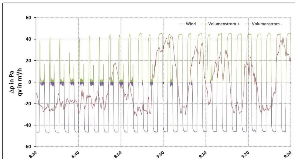
Figure 8: Effective wind pressure (red), volume flow measured via the orifice in delivery direction 1 (green) and delivery direction 2 (violet) at operating level 4: 21/3/18, 8.30 to 9.30 a.m.
