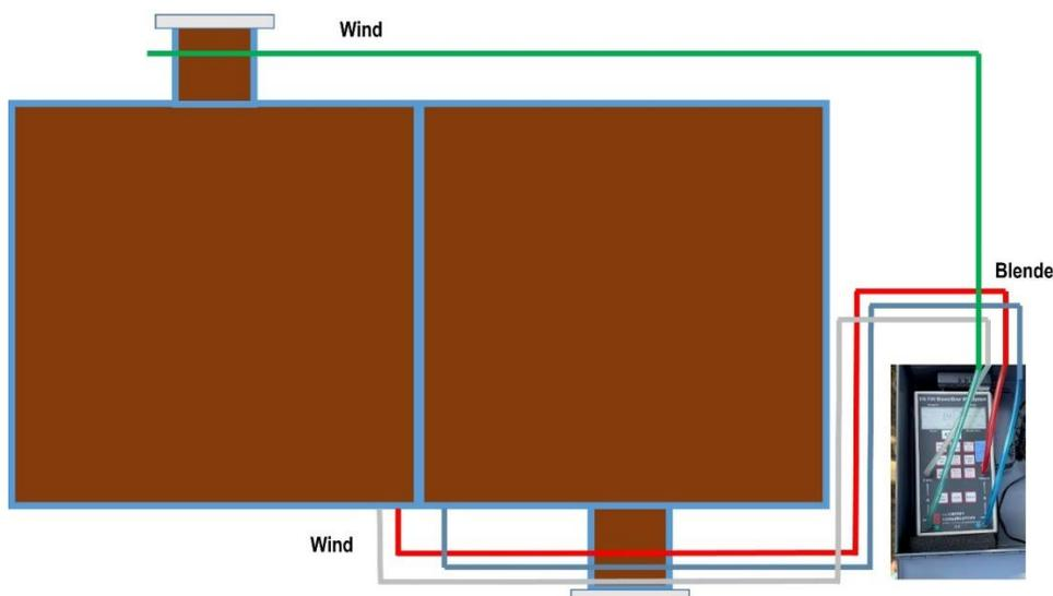
Figure 4: Recording the differential pressures, wind: green-grey, orifice plate: red-blue
