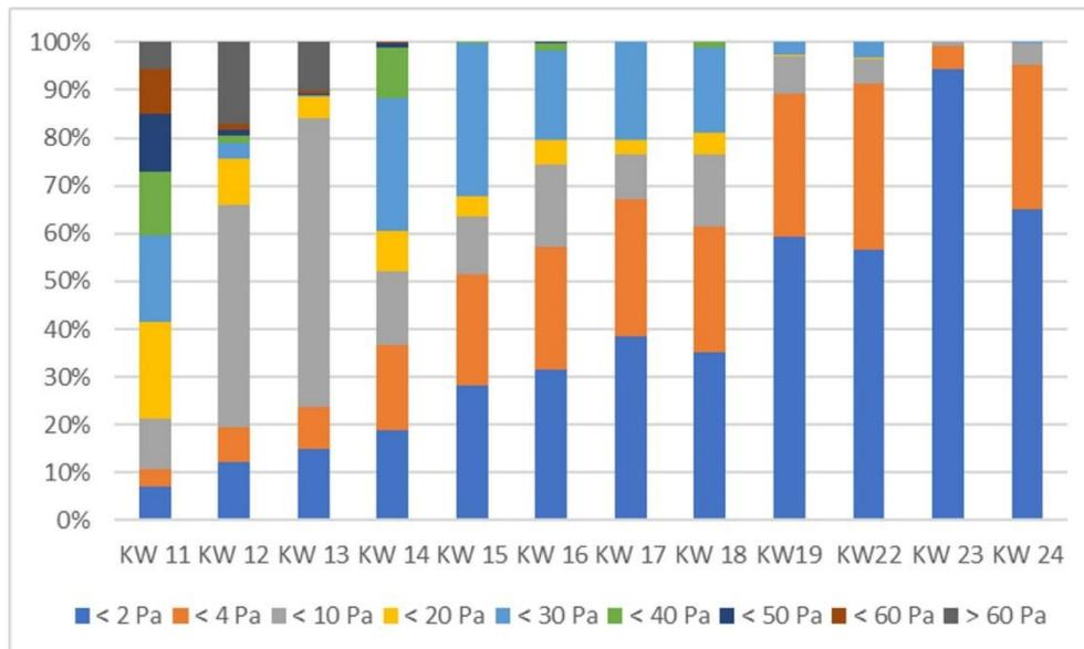
Figure 12: Frequency of absolute wind-induced differential pressures from week 11 (KW 11) to week 24 (KW 24) 2021
