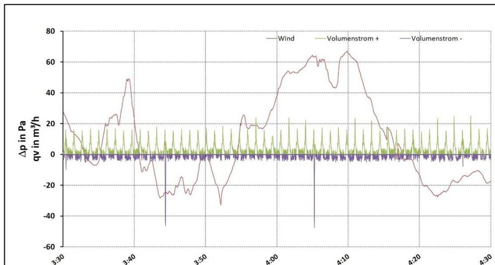
Figure 7: Effective wind pressure (red), volume flow measured via the orifice in delivery direction 1 (green) and delivery direction 2 (violet) at operating level 4: 21/3/18, 3.30 to 4.30 a.m.
