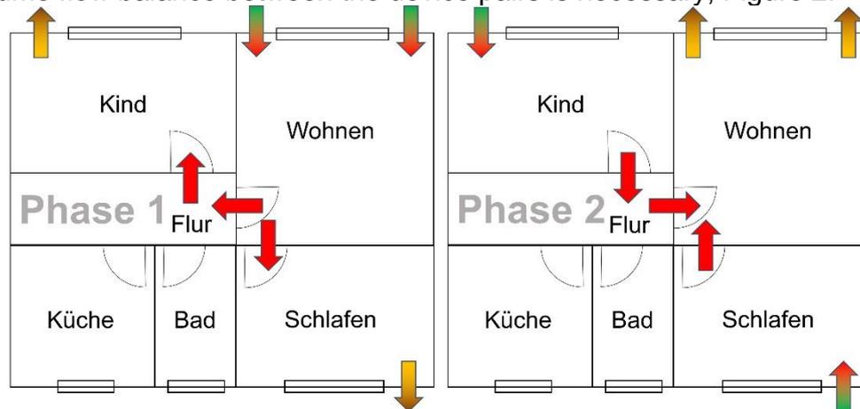
Figure 2: Ventilation phases of push-pull ventilation units in a 3-room flat, ventilation of kitchen and bathroom via manually opening windows.
