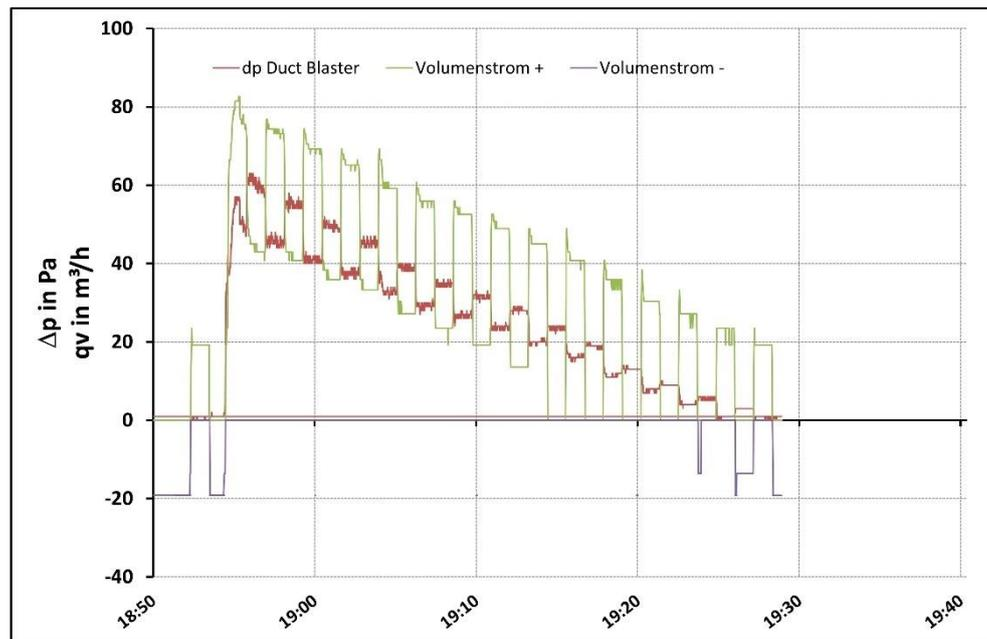
Figure 17: Volume flow under simulated wind pressure: Level 2,  $q_{v,target} = 21 \text{ m}^3/\text{h}$
