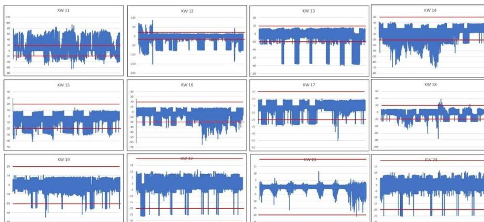
Figure 11: Recording of wind pressure from week 11 (KW 11) to week 24 (KW 24) 2021 with visualisation of the +/- 20 Pa range
