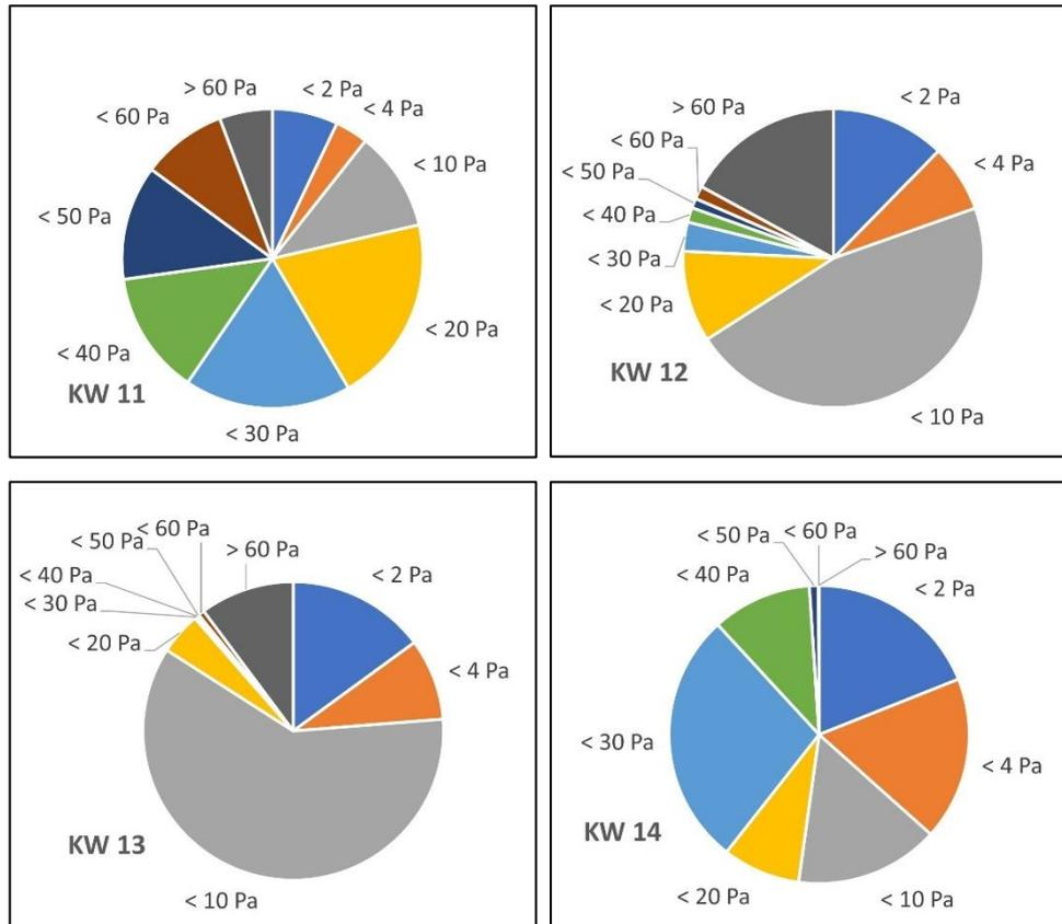
Figure 20: Frequency of wind-induced differential pressures in week 11 (KW 11), week 12 (KW 12), week 13 (KW 13) and week 14 (KW 14)
