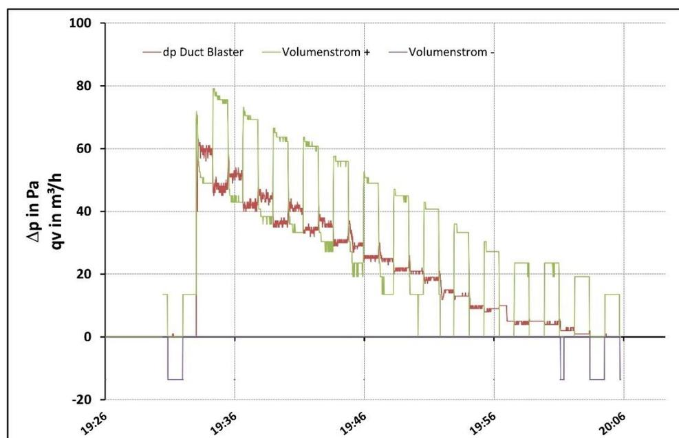
Figure 18: Volume flow under simulated wind pressure: Level 1,  $q_{v,target} = 17 \text{ m}^3/\text{h}$
