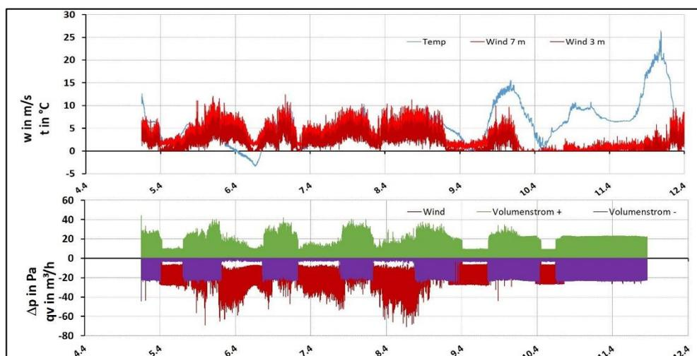
Figure 9: Wind speed at a height of 7 m (light red) and 3 m (dark red), effective wind pressure (red), volume flow measured via the orifice plate in delivery direction 1 (green) and delivery direction 2 (violet) at operating level 3 from 21/4/5 to 21/4/12
