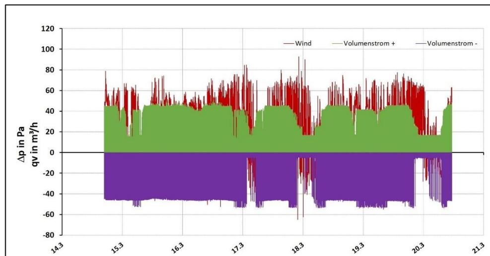
Figure 5: Effective wind pressure (red), volume flow measured via the orifice in delivery direction 1 (green) and delivery direction 2 (violet) at operating level 4: 21/3/15 to 21/3/20
